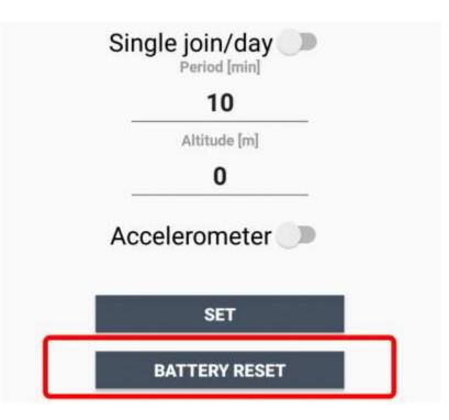
To perform the operation, you need a unique reset code that must be requested to enginko (please provide the DevEUI of the sensor when you ask for that code):
