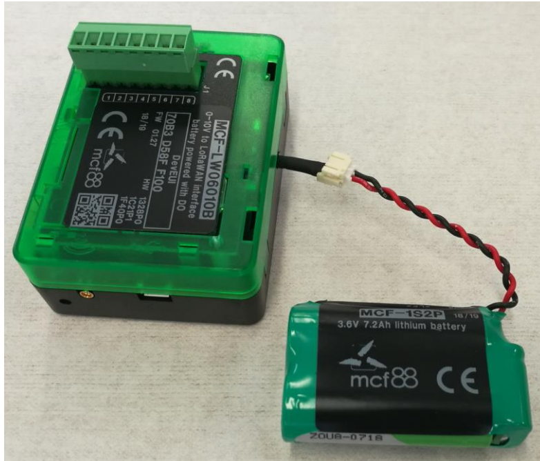
MCF-1S2P 3.6V, 7.2Ah Lithium battery. Current consumption during standby: 18uA.
