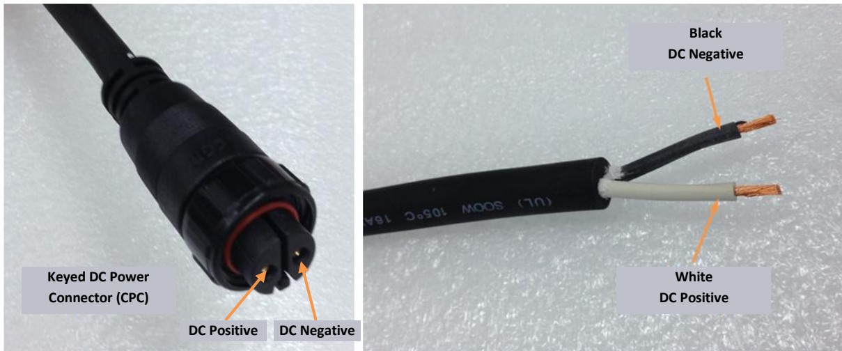
Figure 6: Direct DC Power CPC Connector Connection Polarity
