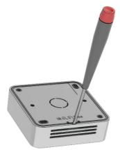
2. Install the batteries. The ERS CO<sub>2</sub> Lite requires one or two AA batteries. The battery type is 3.6V Lithium Battery (ER14505). You can use one battery, but it's recommended that you use two for best performance and battery life. Use battery slot A if only one battery is used.
