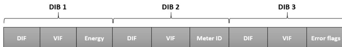
Figure 6: Structure, message format Compact
